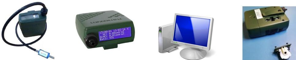
The Industrial Hygienist (IH) connects the DustCount to the PC via Bluetooth and uses the DustCount software to configure the unit prior to running the test. A HEPA filter is used to purge and zero check the initial reading. The alarm threshold is set at 50 ug/m<sup>3</sup> for respirable silica. The IH puts the DustCount on the worker. In this case the DustCount is worn under the protective clothing and the tube is run up to the breathing zone and clipped to the workers lapel.
